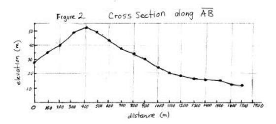
Figure 2 is based on a more complicated landscape that I contoured using a dark pen at a 10 m contour interval and using a lighter pen at a 5 m contour interval. Figure 2 is the cross section along line AB. Each dot represents an elevation number, spaced evenly at 100 m in the horizontal. To walk from A to B, first you climb from an elevation of 28m to a peak of 52 m and then descend to a gradual plain, ending at 12 m elevation 1700 m from your starting point.
